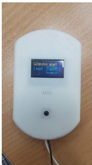
Figure 10. Calcium selective sensor and handy measuring device
